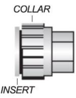
In the event that the fitting ever needs to be removed, you simply turn the collar 1/4 turn counter-clockwise, depress the fitting insert squarely against the fitting to release the teeth, and pull out on the pipe.
