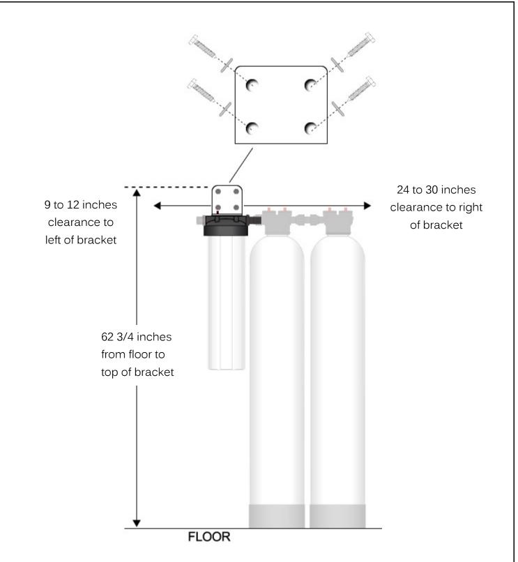
If mounting to drywall, we recommend that you use suitable wall anchors or that you mount a small piece of 3/4 inch plywood to the wall first, ensuring that it is securely screwed into the wall studs. When the cartridge filter housing is full of water, it is heavy, so it is important to ensure that the mounting will be strong enough to support the weight.
