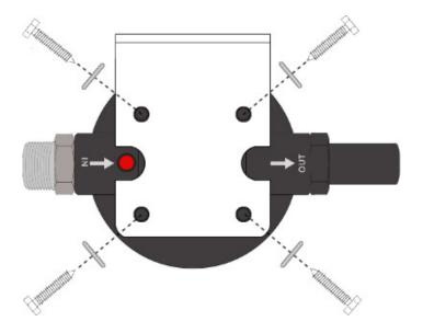
Step 5. - Attach Housing Cap to Wall
