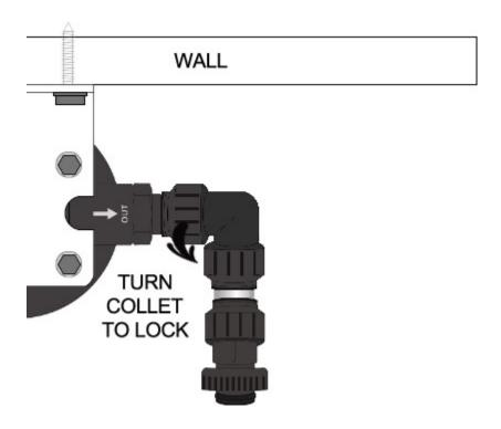
Step 10. - Connect Bypass to Inlet Assembly
