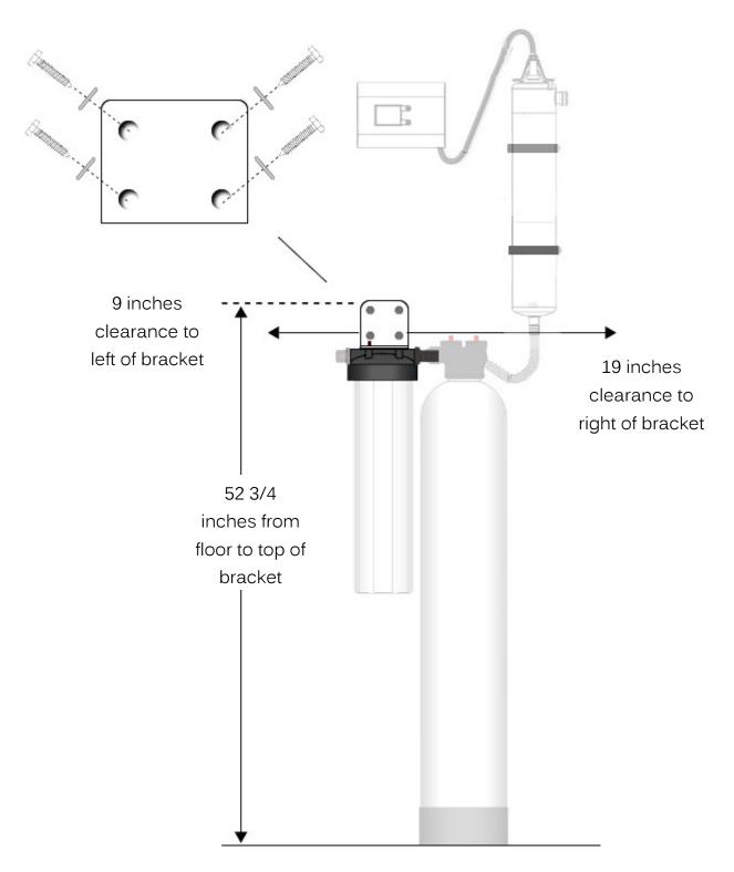
Attach the cartridge filter housing cap and mounting bracket to your wall using the remaining four (4) lag bolts and washers as shown below. The top of the mounting bracket should be mounted EXACTLY 52 3/4 (52.75) inches off the floor. Use a carpenter's
